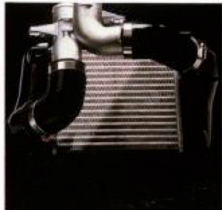
Intercooler provides significant increase in intake charged density for more power
