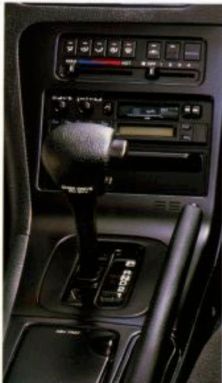
Electronically controlled 4-speed automatic with lockup torque converter and overdrive
