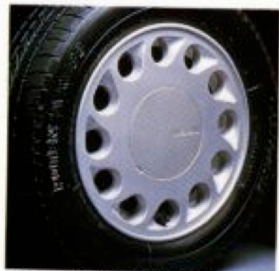
6J-15 alloy wheels fitted with 60 Series tyres
